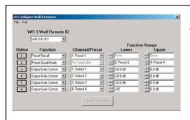
The 24.24M can be configured to be controlled by up to four separate WR-3 Wall remotes. The WR-3 select buttons can be mapped to one of six functions including Preset Recall, Preset Scroll, Input Gain Control, Output Gain Control, Input Mute Control and Output Mute Control. Configuration data is stored in the 24.24M and not in the WR-3.
